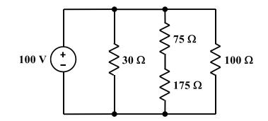
How much power is the 75  $\Omega$  resistor absorbing?
